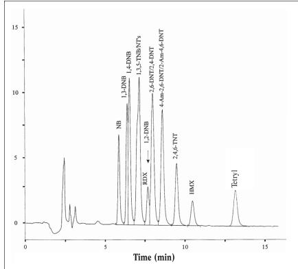
**Figure 3.** LC–CN chromatogram for method 8330 analytes with an eluent composed of water–MeOH–ACN (65:12:23, v/v/v) at 1.2 mL/min. Retention times for surrogate compounds 1,2-DNB and 1,4-DNB are also indicated.
