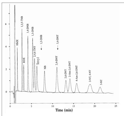
**Figure 1.**  $LC_8$  chromatogram for method 8330 analytes with an eluent composed of water–isopropanol (82:18, v/v) at 1.0 mL/min. Retention times for surrogate compounds 1,2-DNB, 1,4-DNB, and 3,4-DNT are also indicated (although no chromatographic peaks are present for 1,2-DNB and 3,4-DNT).
